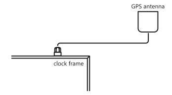
3. Presuming the good position of the GPS receiver the synchronization takes place in approx. 10 to 20 minutes.
