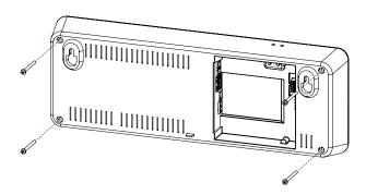
Step 1 – Remove four screws from the back side of the frame.
