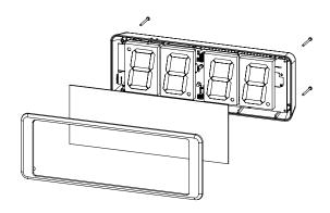
Step 2 – Remove the front frame and the plexiglass.
