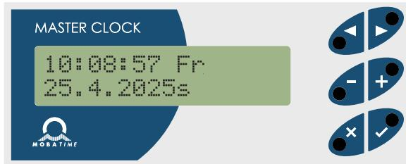
In the Basic Mode, you can scroll through the information screens on the LCD display.
